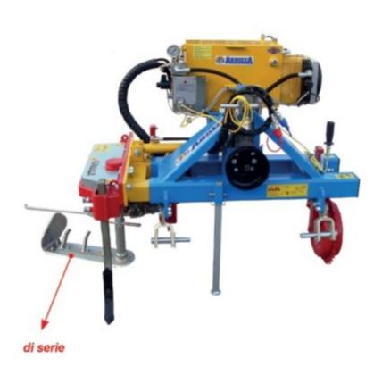
Tool-carrier with hydraulic widening
