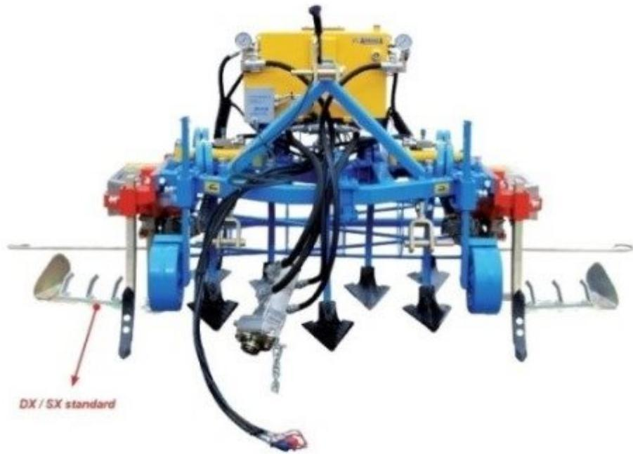
Cultivator with 30x30 spiral spring and cage roller
