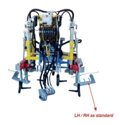
Cultivator with hydraulic side widening, central spring with reversible ploughshares and sides fins, 2 front ramps with reversible ploughshares and external fins
