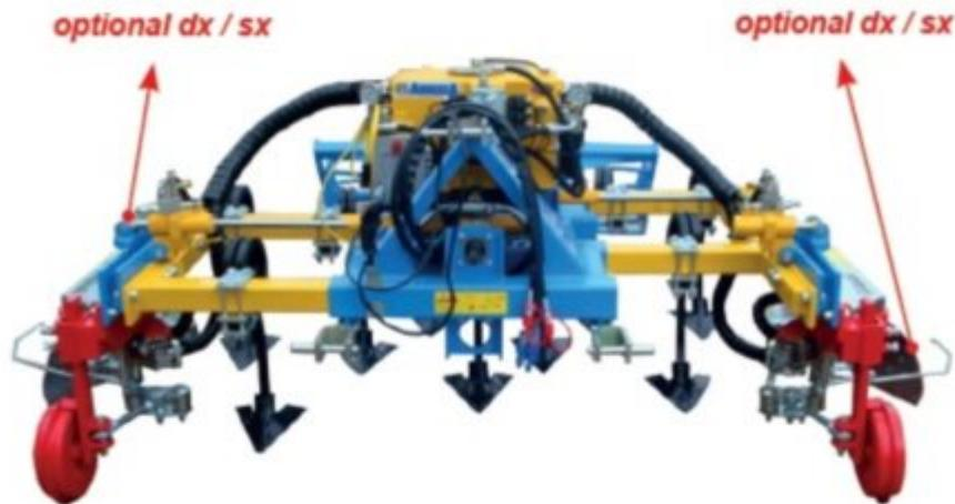
Cultivator with hydraulic widening, 30x30 loop springs with releasable rods and cage roller
