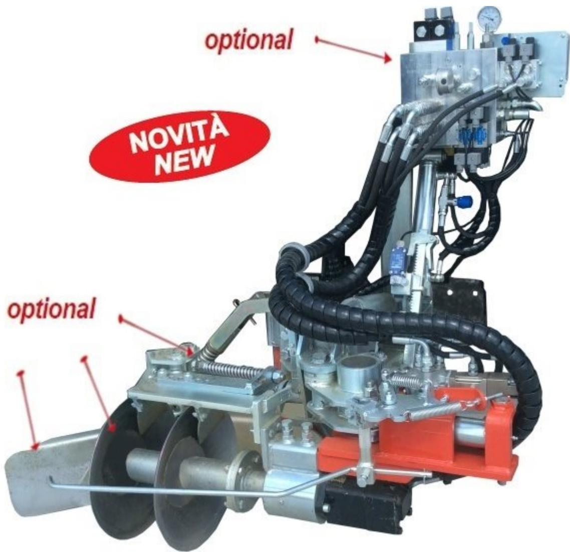
RH inter-row ventral kit alimented by tractor hydraulic system with lifting parallelogram system controlled by multifunction joystick and endowed with double effect cilinder with adjustable electrohydraulic ascent and descent end of stroke system
