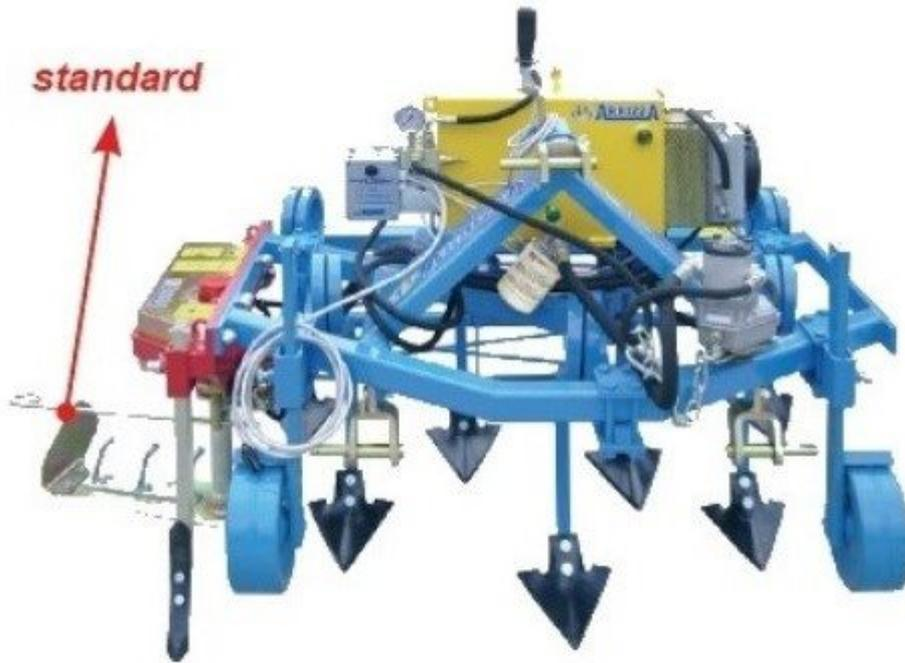
Cultivator with 30x30 spiral spring and cage roller
