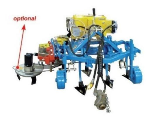
Cultivator with 30x30 spiral spring and cage roller
