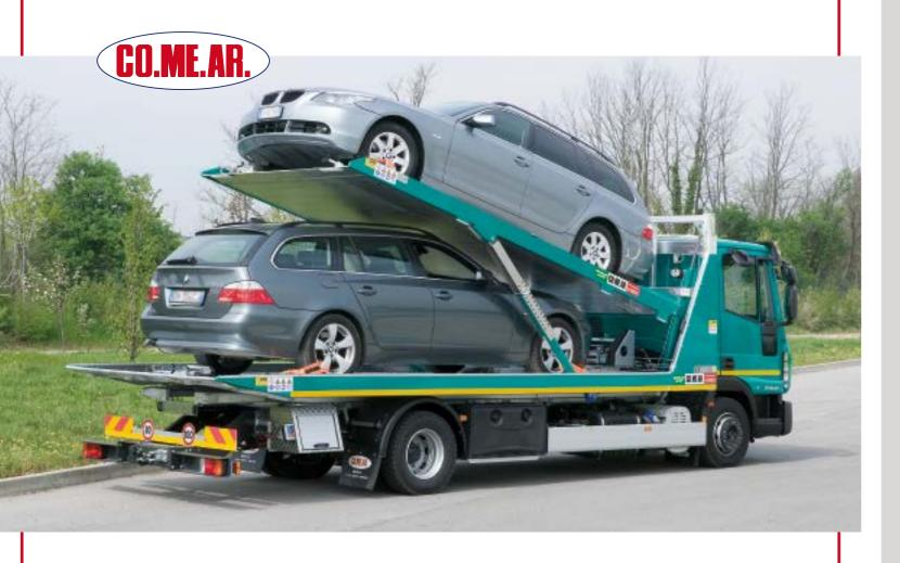
The **DPV 200** is designed for cab trucks with a total minimum ground weight of 10,000 kg. It can transport more than one vehicle. It offers high level of stability during transportation, which is guaranteed by its special structural design featuring a particularly low subframe.
