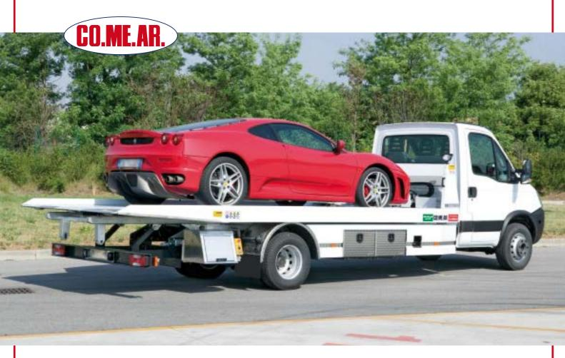
The **SETAL 200** is designed for cab trucks with a total minimum ground weight of 6500 kg and is
