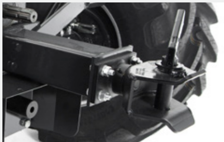
Rear drawbar hitch approved up to 5.000 kg.
