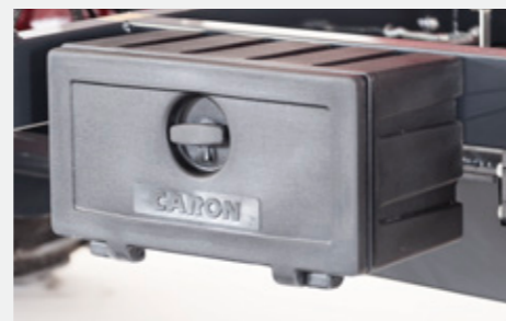
Toolbox placed under the loading platform
