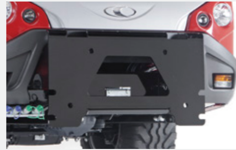
Hydraulic version with front outlets to apply equipment on the fixing plate
