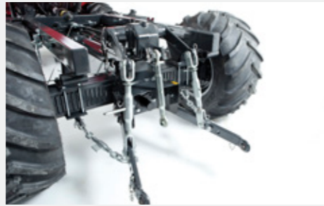
S Rear 3-points linkage system with 500 kgm lifting torque
