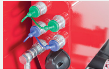
Hydraulic distributor with 3 remote levers, flow rate control and 5 outlets rear the cab
