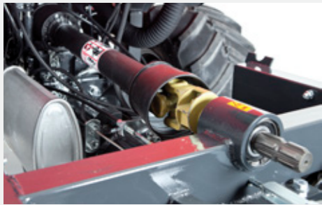
P~ Central PTO with independent hydraulic clutch and electro-hydraulic control, 540 rpm
