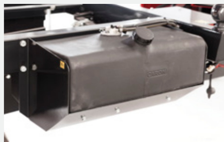
Plastic tank with metal protection support
