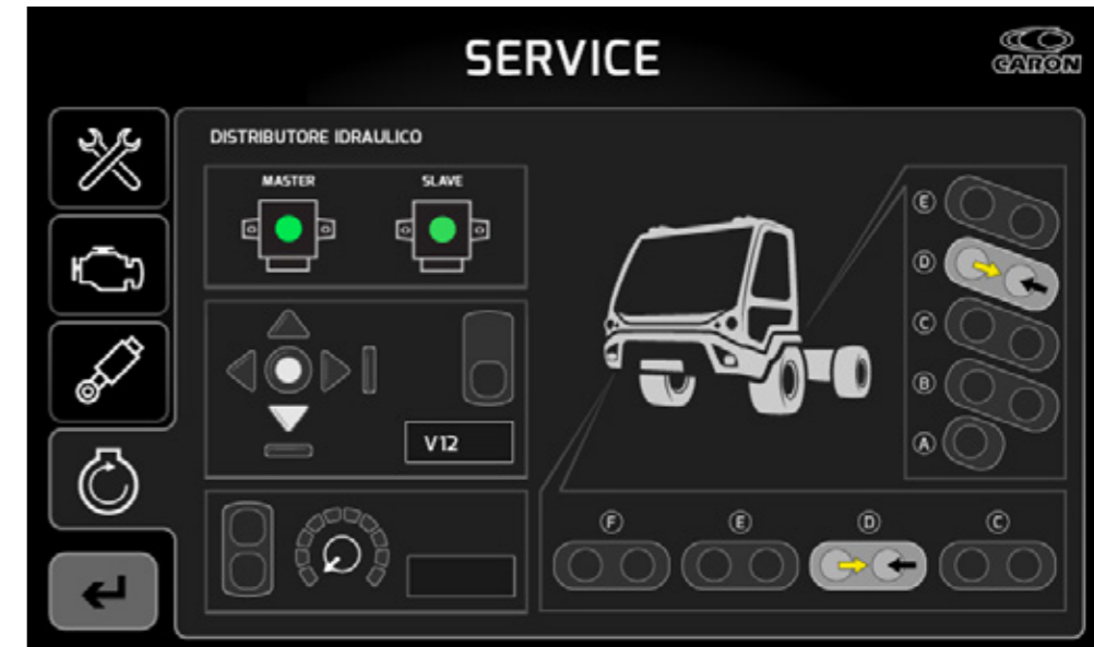
The display's section dedicated to the hydraulic distributor views the control movements, the operating of the relevant electro-valves and the effect of the elements.
