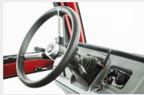
P The column steering wheel can be manually adjusted (height and inclination)
