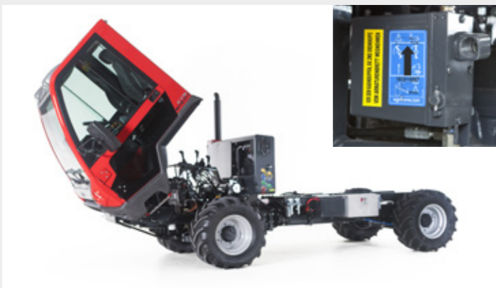
The new dumping system of the cab allows an easier and faster maintenance. Thanks to a hydraulic piston, the cab can be manually dumped in a few seconds without tools.
