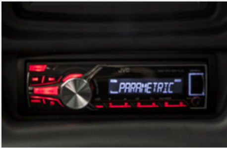
Radio DAB with MP3 Reader and USB inlet. Audio system with two speakers
