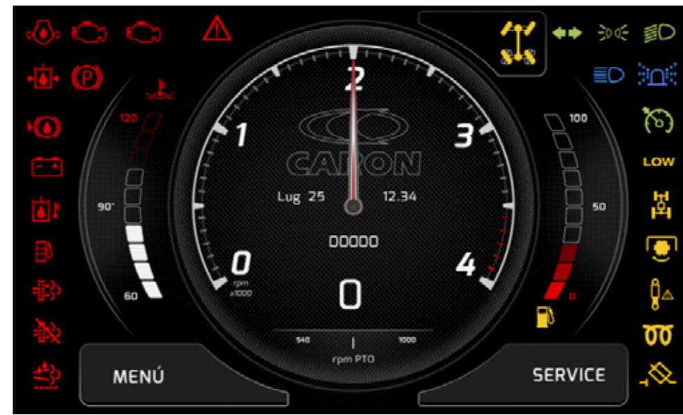
The new 7" digital touch screen display provides all the information for the proper use and maintenance of the vehicle.
