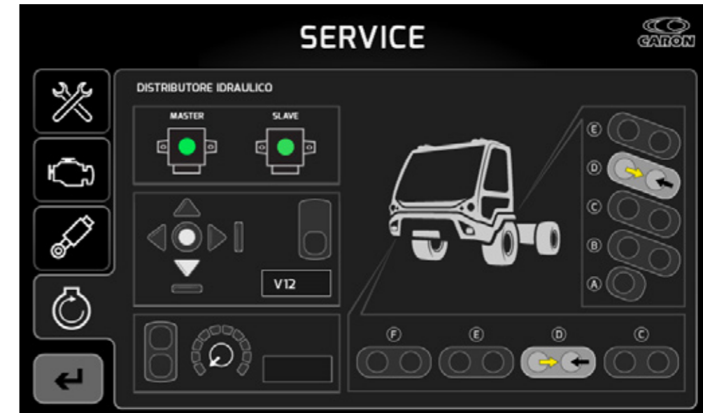
The display's section dedicated to the hydraulic distributor views the control movements, the operating of the relevant electro-valves and the effect of the elements.
