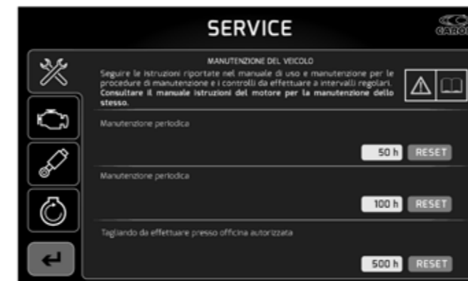
The display provides the operator with further useful information, such as reminders about maintenance operations, fuel consumption, information about engine and suspension system. Available also the pairing with the rear wireless camera.
