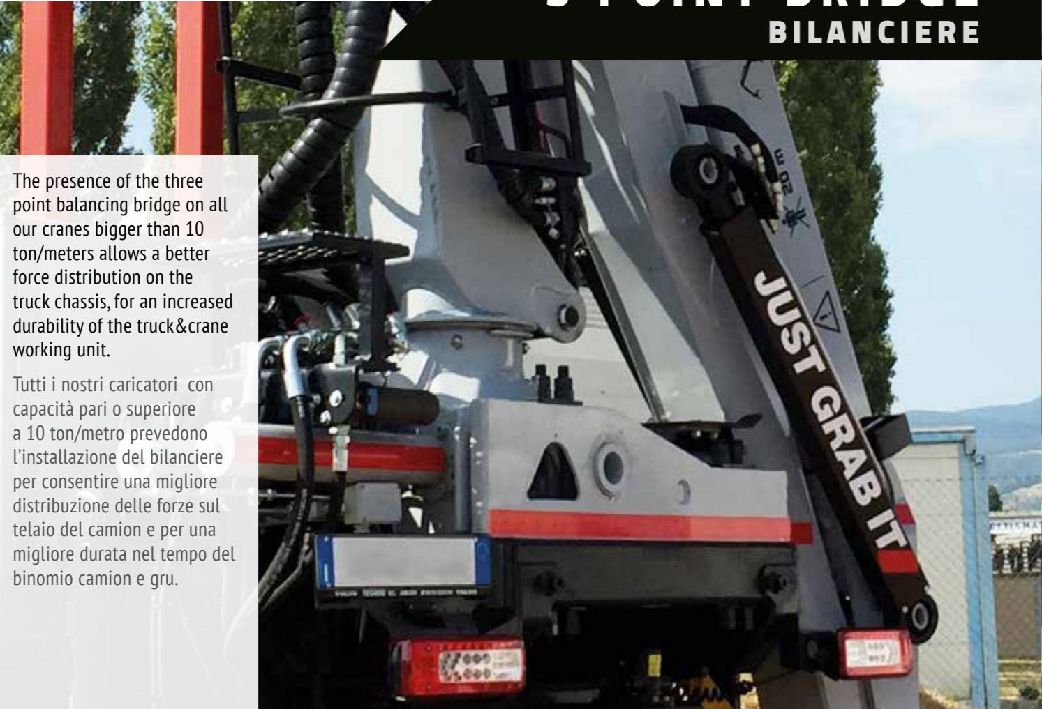
The presence of the three point balancing bridge on all our cranes bigger than 10 ton/meters allows a better force distribution on the truck chassis, for an increased durability of the truck&crane working unit.
