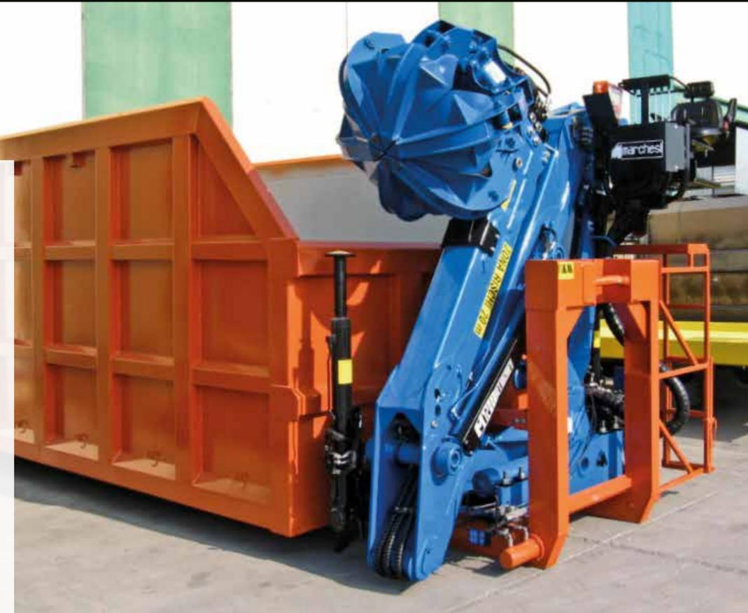
Telescopic first boom has a great outreach thanks to the unique design of our cranes. The protected hydraulic circuit adds value to our products.
