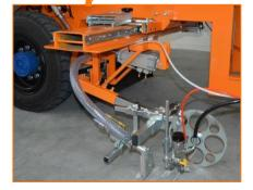
U13 equipped for 2 component Cold Spray Plastic 98:2, internal mixing. With pressurized tank for plastic 500 I, pressurized tank for glass beads 280 I
