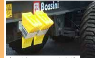
Cunei ferma ruota in PVC PVC wedge stops wheel
