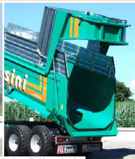
Portellone posteriore maggiorato + cilindri maggiorati Increased rear door with capacity + increased cylinders
