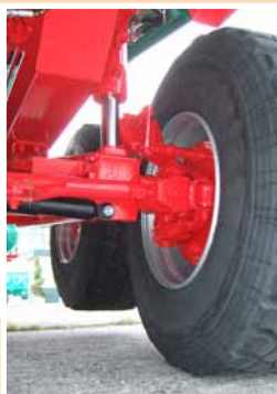
Sospensione brevettata a ruote indipendenti per veicoli a 2 assi Patented wheels independent suspension for vehicles with 2 axles
