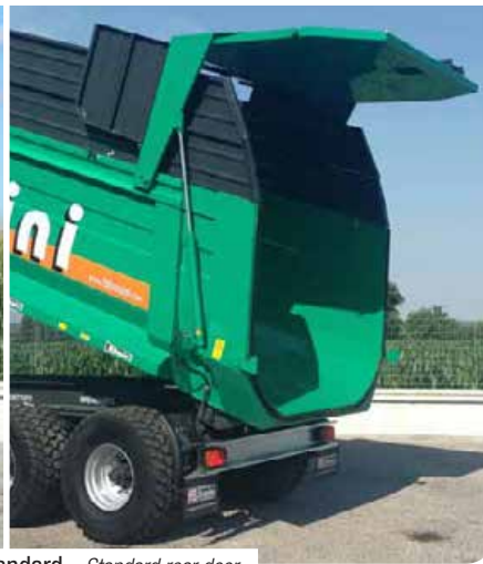
Portellone posteriore standard - Standard rear door
