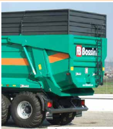
Portellone posteriore maggiorato + cilindri maggiorati Increased rear door with capacity + increased cylinders
