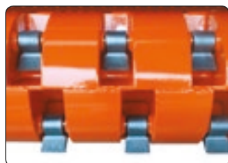
Rotor with forged hammers.
