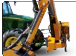
Hydraulic break-back with accumulator controlled autoreset facility.
