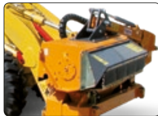
The particular geometry of the arms allows the reach mower positioning in such a way that it does not hinder the visibility during the transfer.
