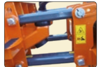
Self levelling device to follow ground contours with 185 mm excursion.
