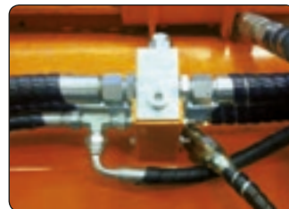
Anti-shock + anti-cavitation valve.
